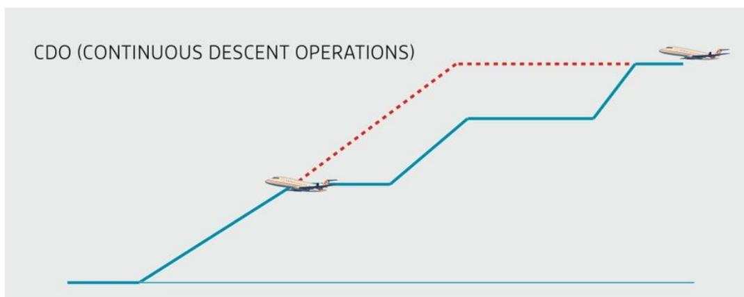
Until now the number of CDO landings was registered manually by the air traffic controllers. The new measuring tool that Belgocontrol uses is based on the analysis of radar data and precisely and automatically detects the landings that are performed in accordance with the CDO procedure. The tool also enables to map aircraft that do not make use of CDO procedures. In the long term a thorough analysis of these data should contribute to reducing the environmental footprint of aviation even more.
